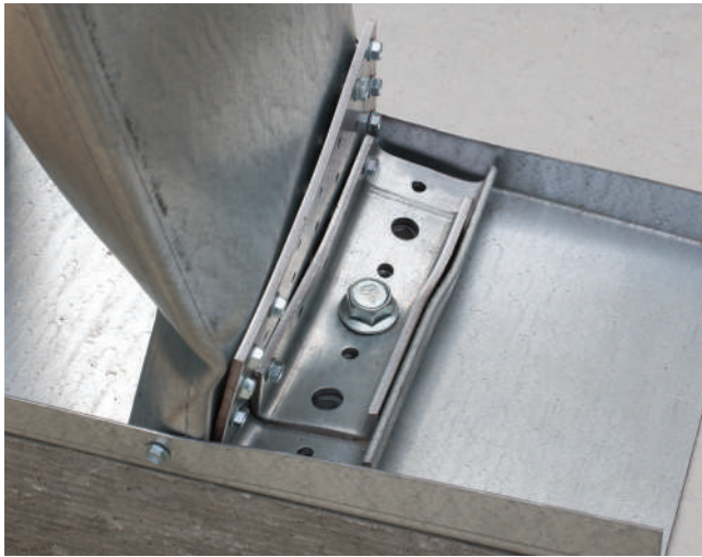
RCKW assembly test with member failure.
